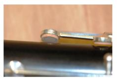
To improve durability, precision, airtight seal and response, very fine pore-free quartz polished aged cork pads and double sealed leather pads are fitted to the top joint,
